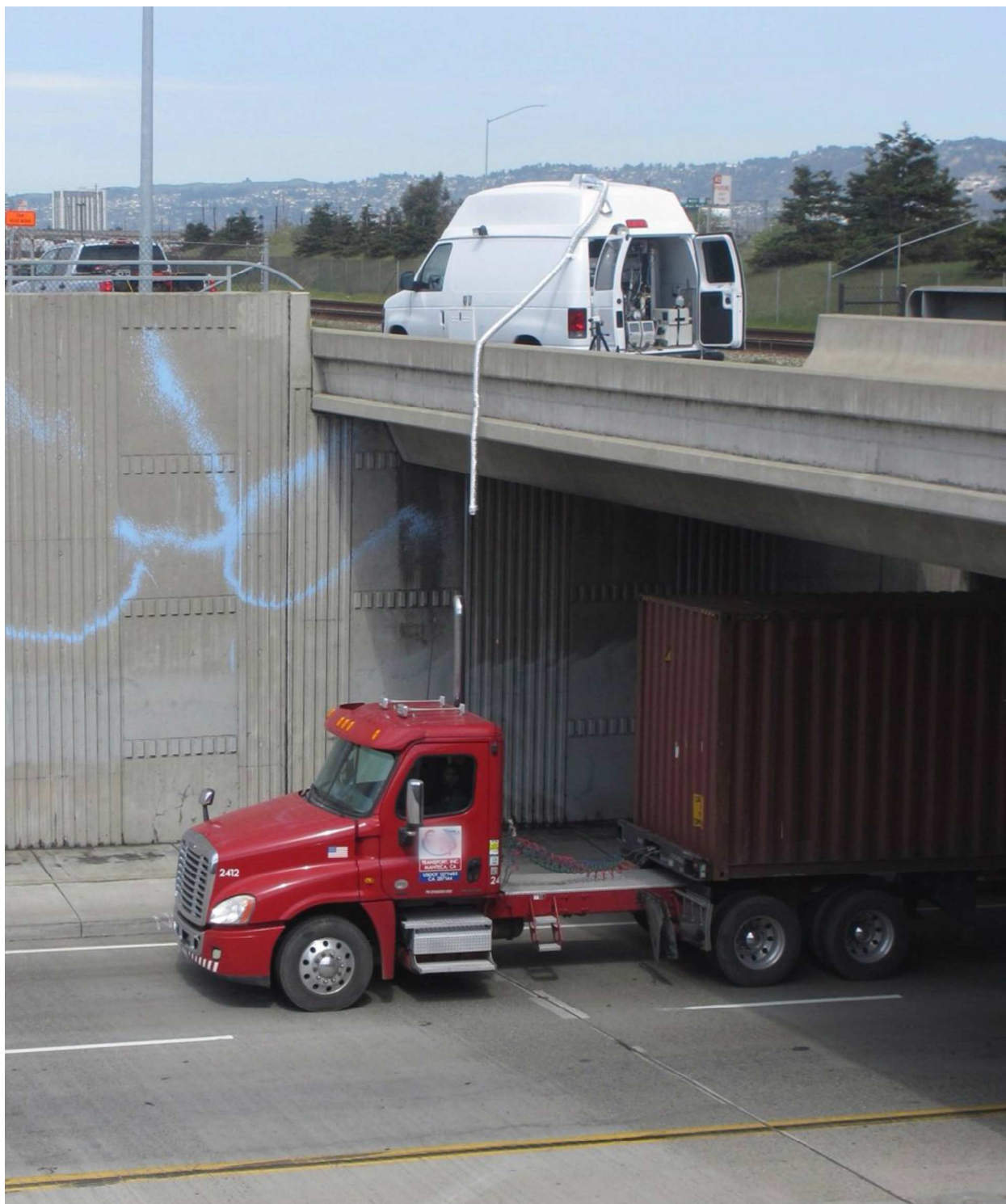
Figure S2. Instrumented van positioned on an overpass sampling the exhaust from a truck en route to the Port of Oakland via a flexible aluminum duct (7.6 cm diameter).
