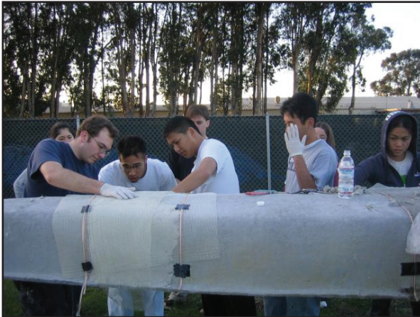
Team Members Attaching Float Rings to Concrete Canoe
