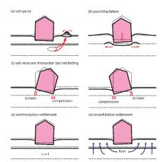
Liquefaction-induced building displacement example (left) and mechanisms (right): (a) ground loss due to soil ejecta; shear-induced settlement from (b) punching failure, or (c) SSI ratcheting; and volumetric-induced settlement from (d) sedimentation or (e) post-liquefaction reconsolidation (Bray and Macedo 2017).
