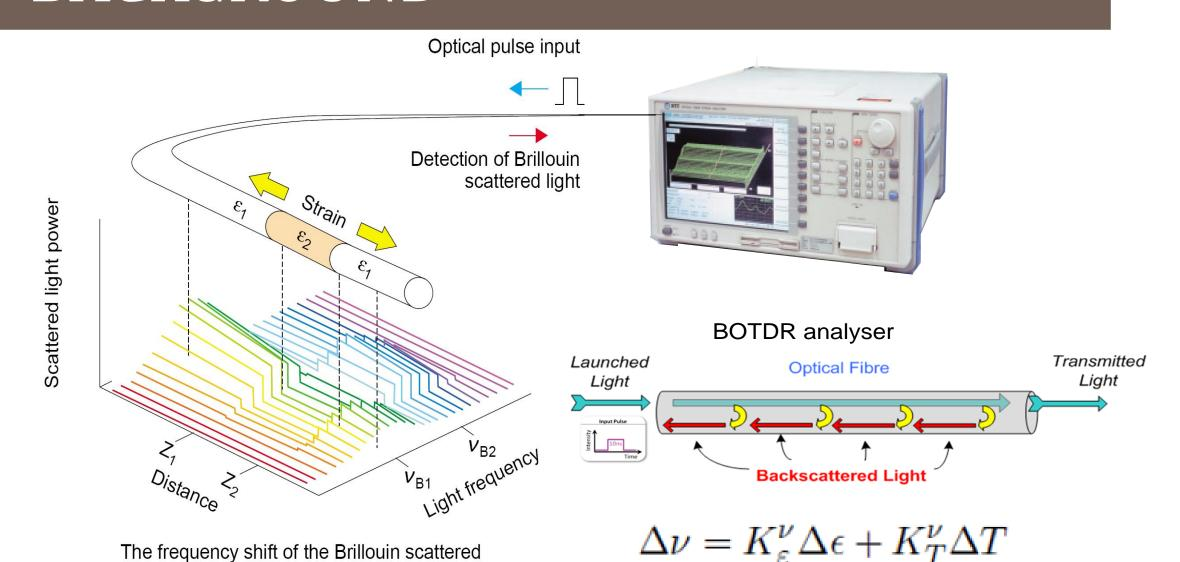
Laser pulse is sent from the analyzer. When the pulse interacts with the acoustic wave on the fiber at different location, a small volume of light will be scatted back with shifted frequency depending on different frequency and energy of the acoustic wave. By examining the shifted frequency, the strain/temperature along the fiber can be monitored.
