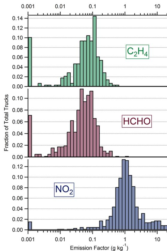
**Figure 3.** Emission factor distributions for ethene, formaldehyde, and nitrogen dioxide.
