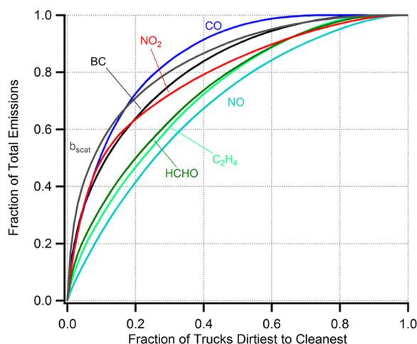
**Figure 5.** Cumulative emission distributions for pollutants measured in heavy-duty truck exhaust plumes. Any  $y$  value on this plot indicates the fraction of total emissions coming from the corresponding highest-emitting fraction ( $x$ ) of all on-road trucks.
