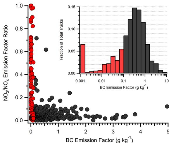
**Figure 1.** Relationship between NO<sub>2</sub>/NO<sub>x</sub> emission ratio and BC emission factor. Each data point represents a single truck, red points correspond to trucks with BC emission factor <0.1 g kg<sup>-1</sup>. Insert plot shows BC emission factor distribution.
