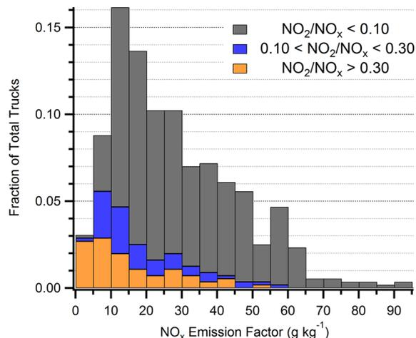
**Figure 2.** NO<sub>x</sub> emission factor distribution with associated ranges of NO<sub>2</sub>/NO<sub>x</sub> emission ratio.
