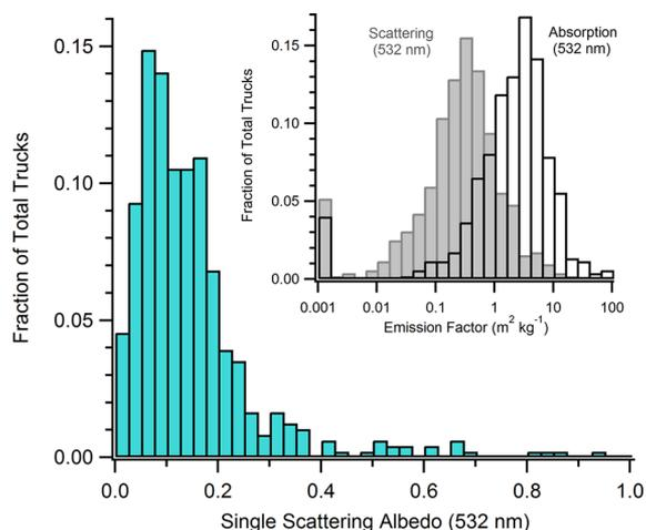
**Figure 4.** Distribution of single scattering albedo for PM emissions from individual trucks, with underlying emission rates of light-scattering and light-absorbing particles (insert plot).
