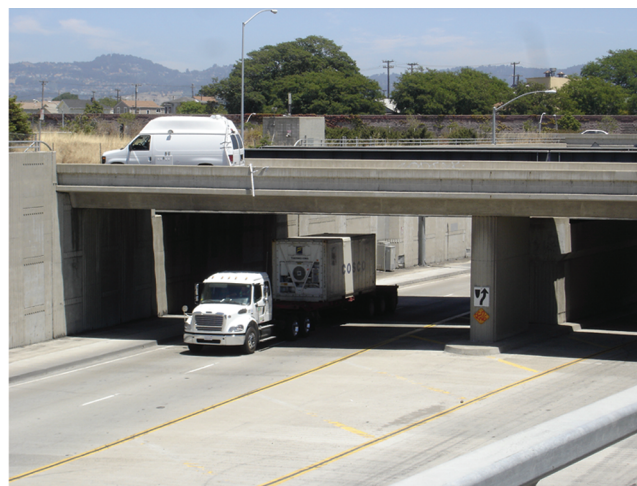
Figure 2. Mobile laboratory parked on Bay Street overpass. Air sampling inlet is positioned above the vertical exhaust stacks of diesel trucks driving westbound on 7th Street toward the Port of Oakland.
