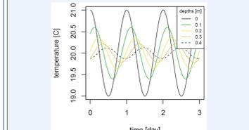
Idealized timeseries used for the synthetic case study. 0 and 0.4m depths are used as boundary conditions of the model, the other timeseries are used in the inversion.
