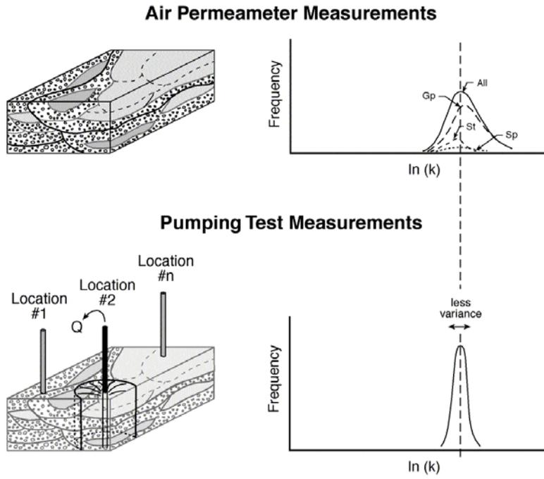
**Fig. 5** Comparing measurements from small and large support scales. From Ritzi *et al.* (2002).
