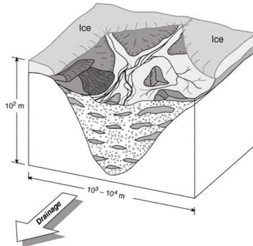
**Fig. 2** Depositional environments in the creation of buried-valley aquifers (from Ritzi *et al.*, 2000).
