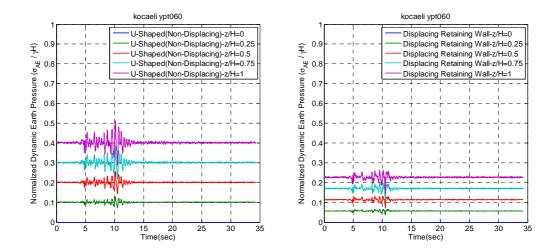
**Figure A.55.** Total earth pressure time series interpreted from strain gage data on both non-displacing and displacing retaining walls for Kocaeli-YPT060-1 for ROOZ02.
