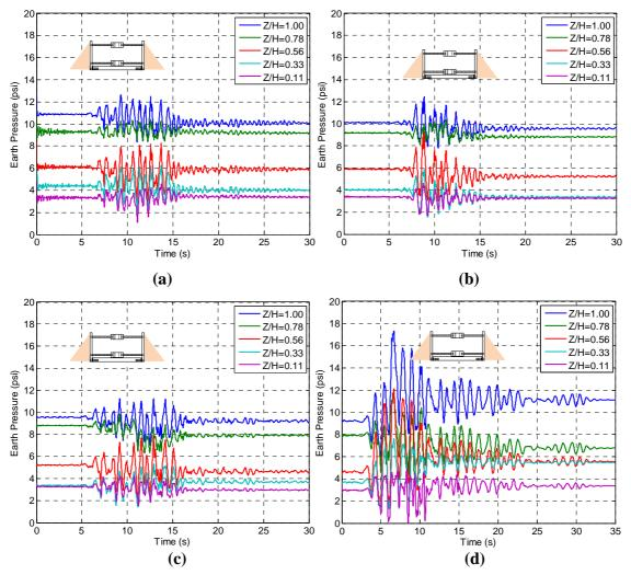
**Figure 5.14.** Total earth pressure time series computed by FLAC on South side of Stiff Basement wall during (a) Kocaeli-YPT330-2, PGA<sub>ff</sub>=0.41 (b) Loma Prieta-WVC270-1, PGA<sub>ff</sub>=0.49 (c) Kocaeli-YPT330-3, PGA<sub>ff</sub>=0.51 and (d) Kobe-TAK090-2, PGA<sub>ff</sub>=0.72.
