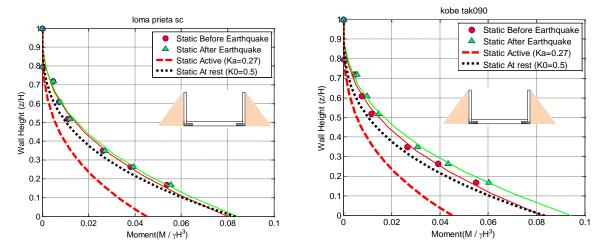
**Figure 4.13.** Normalized static moment profiles measured by the strain gages and estimated using static at-rest and static active pressure distributions of non-displacing cantilever wall before and after Loma Prieta-SC-2, and Kobe-TAK090-2 for ROOZ02.
