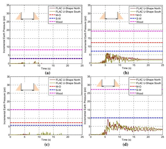
**Figure 5.22.** Incremental earth pressure time series computed by FLAC on Non-Displacing Cantilever wall during (a) Kocaeli-YPT330-1,  $PGA_{ff}$ =0.26 (b) LomaPrieta-SC-1,  $PGA_{ff}$ =0.62 (c) LomaPrieta-SC-2,  $PGA_{ff}$ =0.48 and (d) Kobe-TAK090-1,  $PGA_{ff}$ =0.87.
