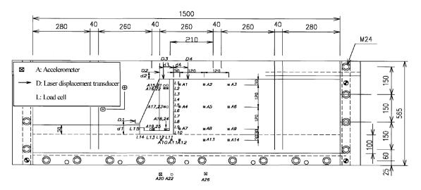
Figure 2.10. Nakamura (2006) test configuration.
