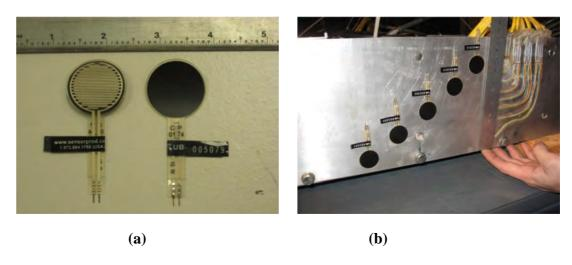
**Figure 3.20.** (a) The Tactilus free form pressure transducer (b) pressure transducers placed on the sides of retaining structures.
