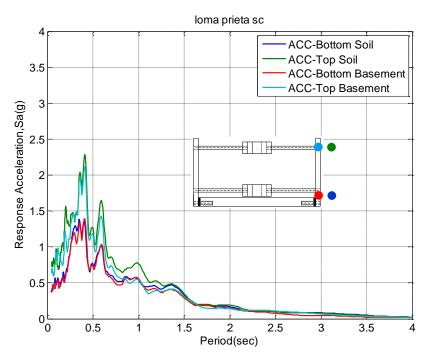
**Figure 4.7.** Spectral accelerations of top and bottom of the soil and the basement structure for Loma Prieta-SC-2 event (5% damped).
