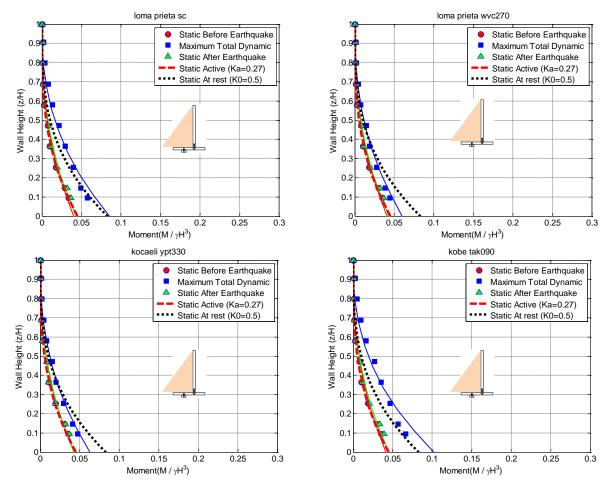
**Figure 4.16.** Maximum total wall moment profiles measured by strain gages and static active and at rest moment estimates on the displacing retaining wall for Loma Prieta-SC-2, Loma Prieta-WVC270-2, Kocaeli-YPT330-2 and Kobe-TAK090-2 for ROOZ02.
