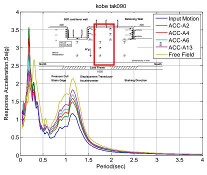
**Figure 4.4.** (a) Spectral accelerations at different elevations in ROOZ02 for Kobe-TAK090-2 event (5% damped).
