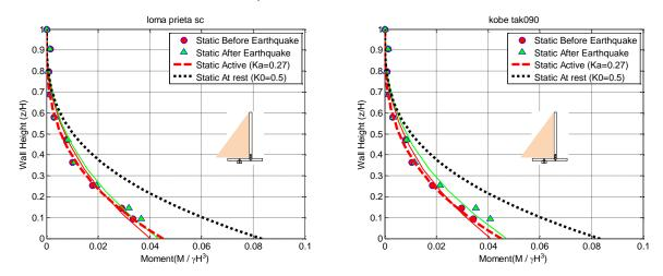
**Figure 4.14.** Normalized static moment profiles measured by the strain gages and estimated using static at-rest and static active pressure distributions of displacing retaining wall before and after Loma Prieta-SC-2, and Kobe-TAK090-2 for ROOZ02.
