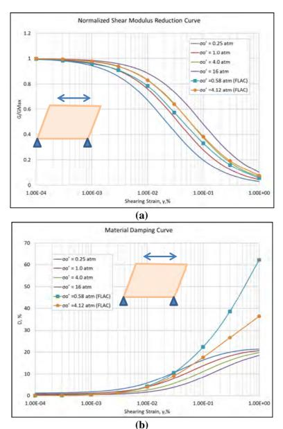
**Figure 5.6.** (a) Modulus reduction and (b) Damping ratio curve estimated by FLAC using UBCHYST model.
