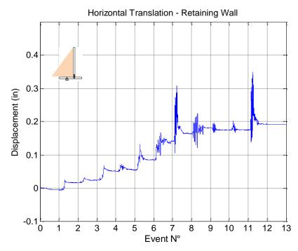
Figure 4.27. Horizontal translation of the displacing retaining wall during shaking evens.
