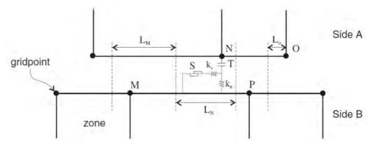
Figure 5.3. Schematic of the FLAC interface element (from Itasca 2011).
