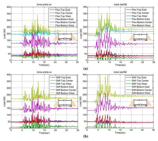
**Figure 4.19.** Total lateral force time series estimated by load cells on both stiff and flexible non-displacing basement walls for Loma Prieta-SC-1 and Kobe-TAK090-2 for ROOZ01 (a) flexible basement wall (b) stiff basement wall.
