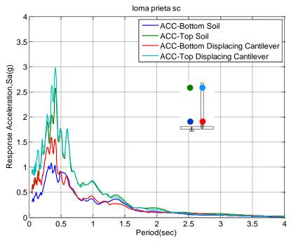
**Figure 4.11.** Spectral accelerations of top and bottom of the soil and displacing retaining wall for Loma Prieta-SC-2 event (5% damped).
