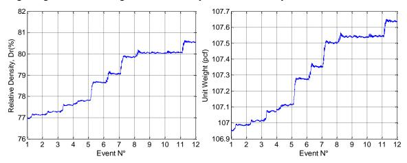
**Figure 4.2.** Soil settlement and relative density after different shaking events for ROOZ02.
