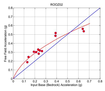
Figure 4.6. Base motion amplification/de-amplification for ROOZ02 experiment.
