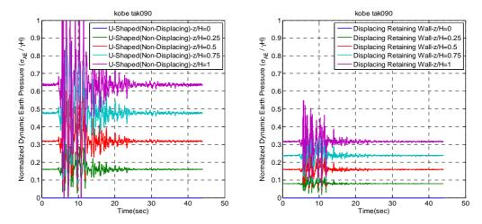
**Figure A.64.** Total earth pressure time series interpreted from strain gage data on both non-displacing and displacing retaining walls for Kobe-TAK090-2 for ROOZ02.
