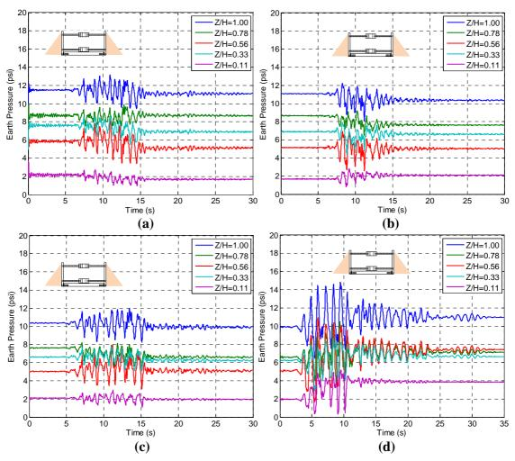
**Figure 5.15.** Total earth pressure time series computed by FLAC on North side of Stiff Basement wall during (a) Kocaeli-YPT330-2, PGA<sub>ff</sub>=0.41 (b) Loma Prieta-WVC270-1, PGA<sub>ff</sub>=0.49 (c) Kocaeli-YPT330-3, PGA<sub>ff</sub>=0.51 and (d) Kobe-TAK090-2, PGA<sub>ff</sub>=0.72.
