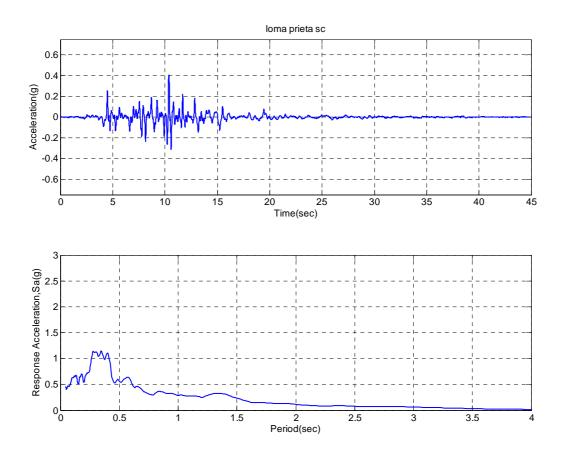
**Figure A.19.** Horizontal acceleration, response spectrum (5% damping) of Loma Prieta-SC-2 input ground motion for ROOZ02.
