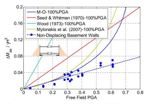
**Figure 6.4.** Maximum dynamic moment increment as a function of PGA for non-displacing basement structures with medium dense sand backfill.
