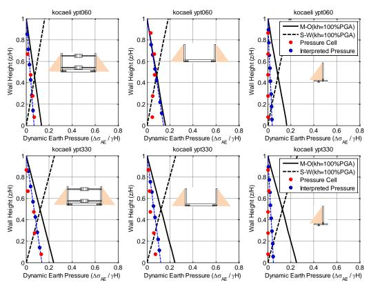
**Figure 4.25.** Dynamic earth pressure distributions directly measured and interpreted from the pressure sensors and strain gage and load cell data and estimated M-O as well as S-W on walls for Kocaeli-YPT060-3 (PGA<sub>ff</sub>=0.25), Kocaeli-YPT330-2 (PGA<sub>ff</sub>=0.34).
