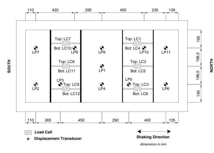
Figure 3.4. ROOZ01 model configuration, plan view (dimension in mm).
