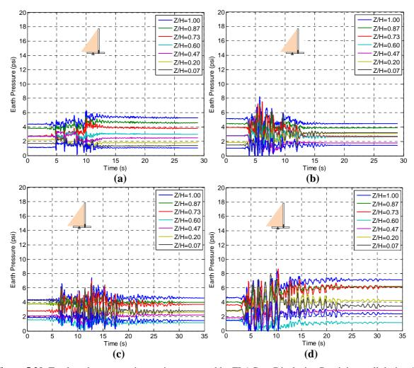
**Figure 5.20.** Total earth pressure time series computed by FLAC on Displacing Retaining wall during (a) Kocaeli-YPT330-1,  $PGA_{ff}$ =0.26 (b) LomaPrieta-SC-1,  $PGA_{ff}$ =0.62 (c) LomaPrieta-SC-2,  $PGA_{ff}$ =0.48 and (d) Kobe-TAK090-1,  $PGA_{ff}$ =0.87.
