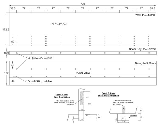
Figure 3.10. Stiff U-shaped model structure configuration (dimensions in mm, model scale).
