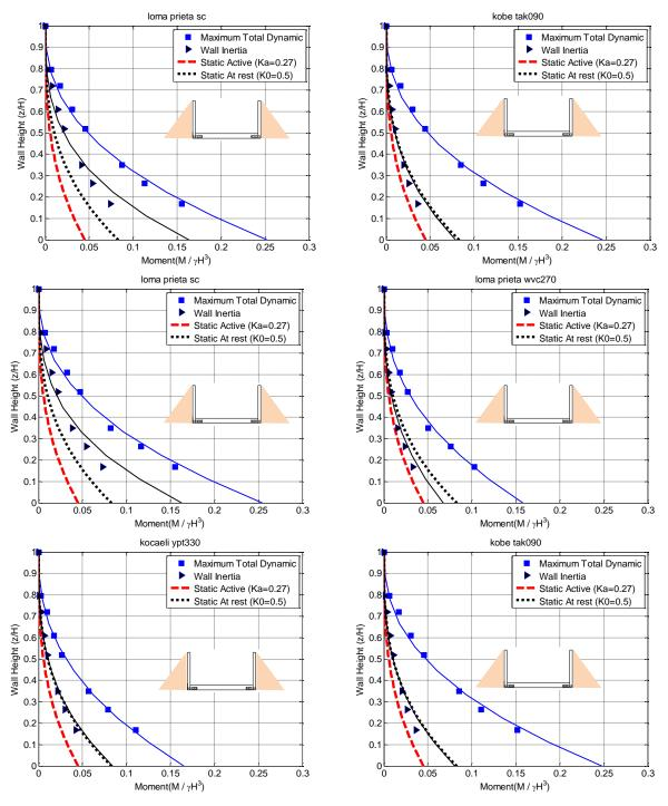
**Figure 4.17.** Maximum total and inertial wall moment profiles measured by strain gages and accelerometers on the non-displacing cantilever wall for Loma Prieta-SC-1, Kobe-TAK090-1, Loma Prieta-SC-2, Loma Prieta-WVC270-2, Kocaeli-YPT330-2 and Kobe-TAK090-2 for ROOZ02.
