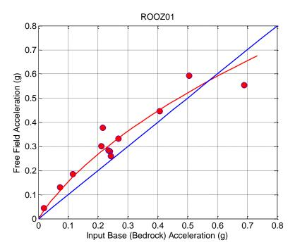
Figure 4.5. Base motion amplification/de-amplification for ROOZ01 experiment.
