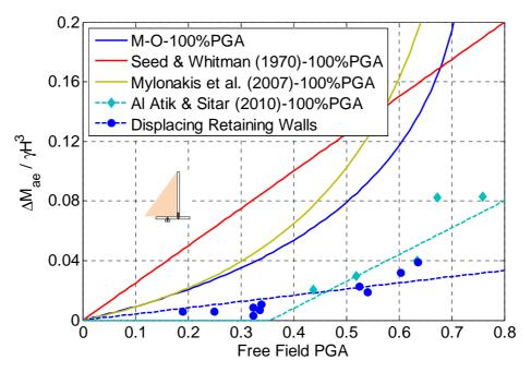
**Figure 6.5.** Maximum dynamic moment increment as a function of PGA for displacing retaining walls with medium dense sand backfill.
