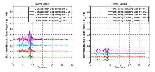
**Figure A.56.** Total earth pressure time series interpreted from strain gage data on both non-displacing and displacing retaining walls for Kocaeli-YPT060-2 for ROOZ02.
