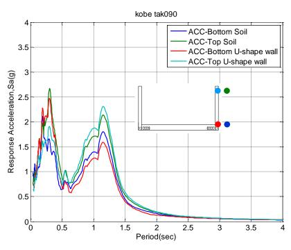
**Figure 4.10.** Spectral accelerations of top and bottom of the soil and the non-displacing cantilever wall for Kobe-TAK090-2 event (5% damped).
