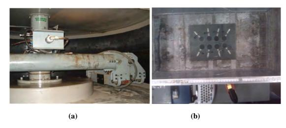
**Figure 3.19.** (a) UC Davis Schaevits centrifuge (1m radius) (b) Tactilus free form sensor placed on the base of small container.
