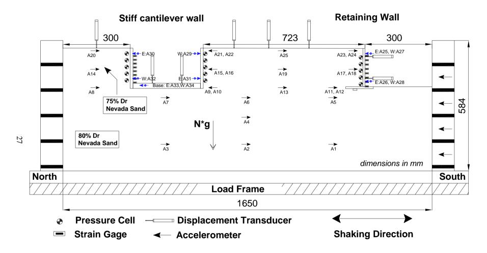
Figure 3.5. ROOZ02 Model configuration, profile view (dimension in mm).
