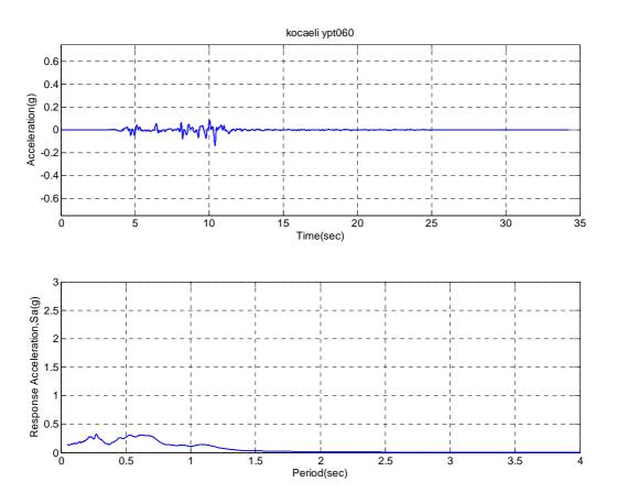
**Figure A.13.** Horizontal acceleration, response spectrum (5% damping) of Kocaeli-YPT060-1 input ground motion for ROOZ02.
