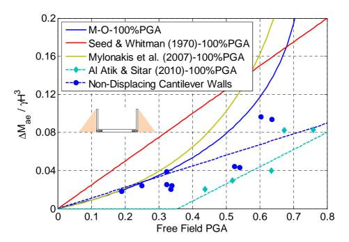
**Figure 6.6.** Maximum dynamic moment increment as a function of PGA for non-displacing U- shaped cantilever walls with medium dense sand backfill.
