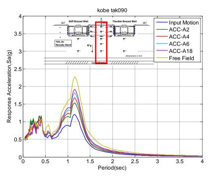
**Figure 4.3.** (a) Spectral accelerations at different elevations in ROOZ01 for Kobe-TAK090-2 event (5% damped).
