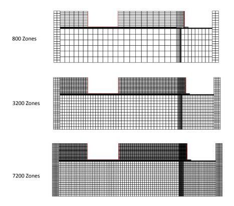
Figure 5.11. FD meshes with different resolutions.
