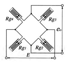
Figure 3.18. Wheatstone Bridge circuit.
