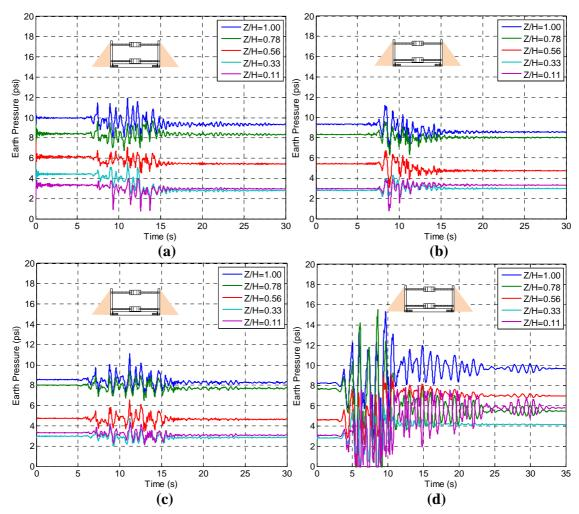
**Figure 5.17.** Total earth pressure time series computed by FLAC on North side of Flexible Basement wall during (a) Kocaeli-YPT330-2, PGA $_{\rm ff}$ =0.41 (b) Loma Prieta-WVC270-1, PGA $_{\rm ff}$ =0.49 (c) Kocaeli-YPT330-3, PGA $_{\rm ff}$ =0.51 and (d) Kobe-TAK090-2, PGA $_{\rm ff}$ =0.72.
