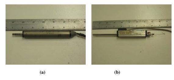
Figure 3.22. Displacement transducers (a) LP (b) LVDT.
