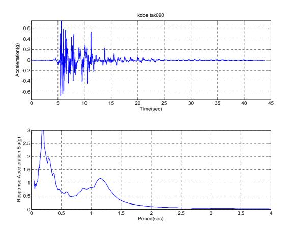
**Figure A.22.** Horizontal acceleration, response spectrum (5% damping) of Kobe-TAK090-2 input ground motion for ROOZ02.
