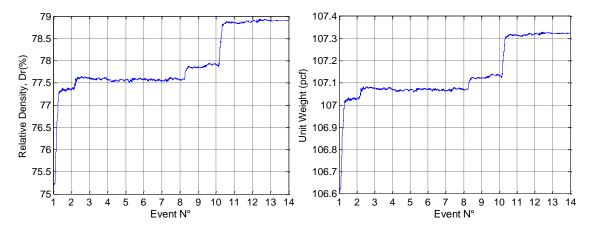
Figure 4.1. Soil settlement and relative density after different shaking events for ROOZ01.
