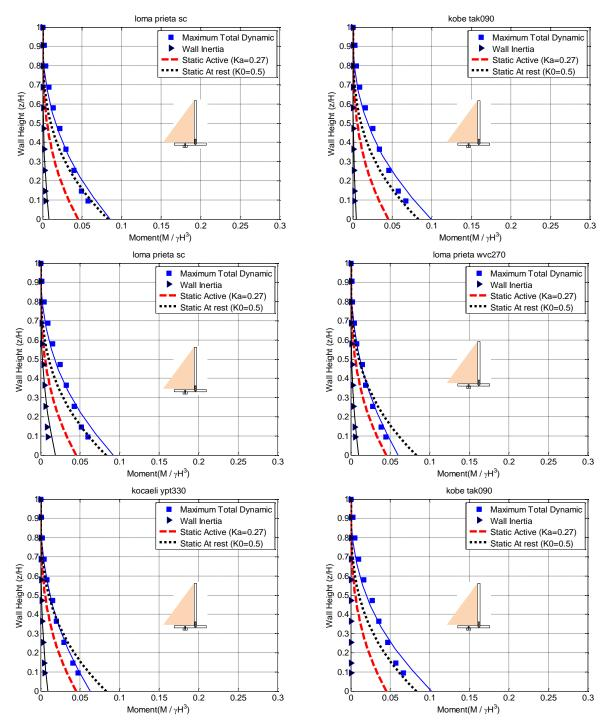
**Figure 4.18.** Maximum total and inertial wall moment profiles measured by strain gages and accelerometers on the displacing retaining wall for Loma Prieta-SC-1, Kobe-TAK090-1, Loma Prieta-SC-2, Loma Prieta-WVC270-2, Kocaeli-YPT330-2 and Kobe-TAK090-2 for ROOZ02.
