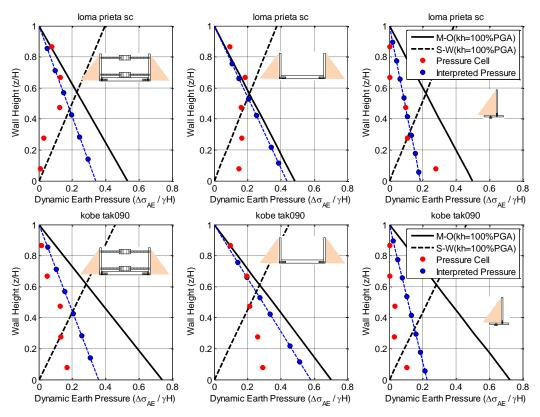
**Figure 4.26.** Dynamic earth pressure distributions directly measured and interpreted from the pressure sensors and strain gage and load cell data and estimated M-O as well as S-W on walls for Loma Prieta-SC-1 (PGA<sub>ff</sub>=0.51), Kobe-TAK090-2 (PGA<sub>ff</sub>=0.61).
