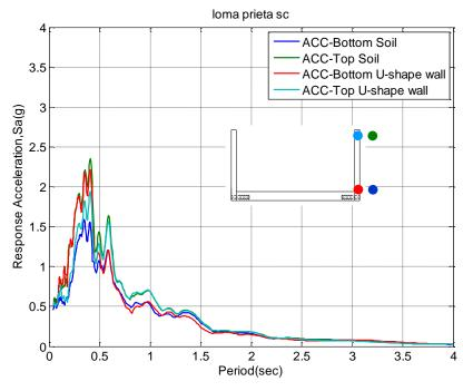
**Figure 4.9.** Spectral accelerations of top and bottom of the soil and the non-displacing cantilever wall for Loma Prieta-SC-2 event (5% damped).
