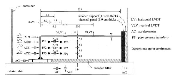
**Figure 2.9.** Dewoolkar (2001) typical test configuration.
