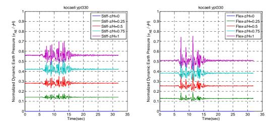
**Figure A.54.** Total earth pressure time series interpreted from load cell data on both stiff and flexible non-displacing basement walls for Kocaeli-YPT330-3 for ROOZ01.
