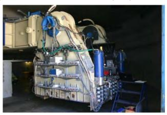
Figure 3.1. The large centrifuge payload bucket at the Center for Geotechnical Modeling at U.C. Davis.
