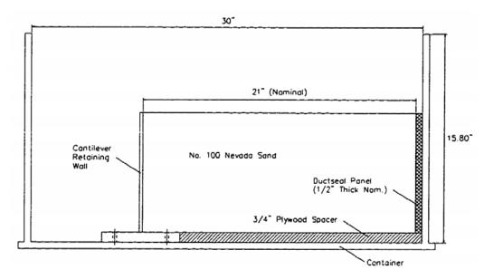
Figure 2.8. Stadler (1996) typical test configuration.
