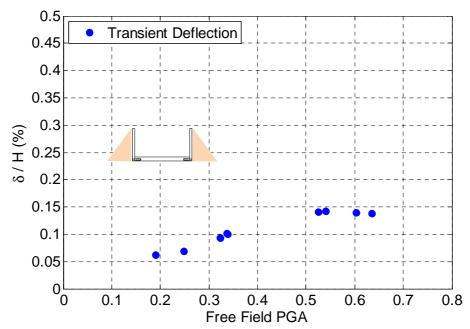
Figure 6.15. Transient deflection of non-displacing retaining wall.
