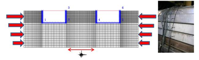
**Figure 7.5.** Apply dynamic excitation to the lateral boundary grid in addition to base of the model to reduce the uncertainty of container behavior during shaking.
