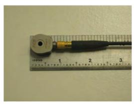
Figure 3.16. PCB Piezotronics acclerometers.
