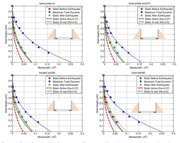
**Figure 4.15.** Maximum total wall moment profiles measured by strain gages and static active and at rest moment estimates on the non-displacing cantilever wall for Loma Prieta-SC-2, Loma Prieta-WVC270-2, Kocaeli-YPT330-2 and Kobe-TAK090-2 for ROOZ02.
