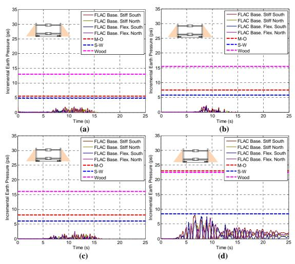
**Figure 5.21.** Incremental earth pressure time series computed by FLAC on South and North sides of Both Stiff and Flexible Basement wall during (a) Kocaeli-YPT330-2,  $PGA_{ff}$ =0.41 (b) Loma Prieta-WVC270-1,  $PGA_{ff}$ =0.49 (c) Kocaeli-YPT330-3,  $PGA_{ff}$ =0.51 and (d) Kobe-TAK090-2,  $PGA_{ff}$ =0.72.
