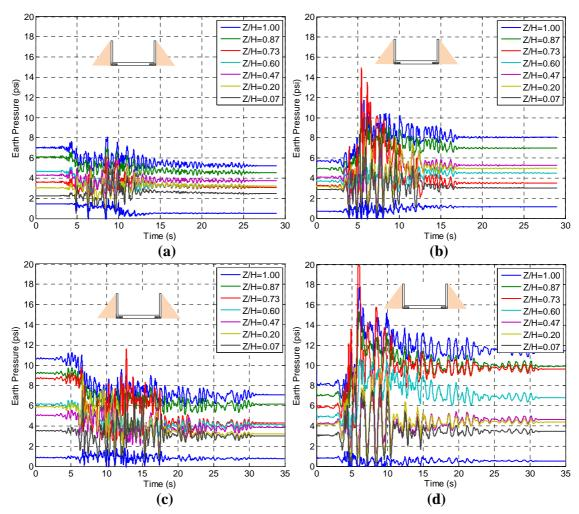
**Figure 5.18.** Total earth pressure time series computed by FLAC on North side of Non-Displacing Cantilever wall during (a) Kocaeli-YPT330-1,  $PGA_{ff}$ =0.26 (b) LomaPrieta-SC-1,  $PGA_{ff}$ =0.62 (c) LomaPrieta-SC-2,  $PGA_{ff}$ =0.48 and (d) Kobe-TAK090-1,  $PGA_{ff}$ =0.87.
