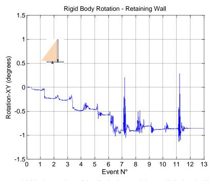
Figure 4.28. Rigid body rotation of the displacing retaining wall during shaking evens.
