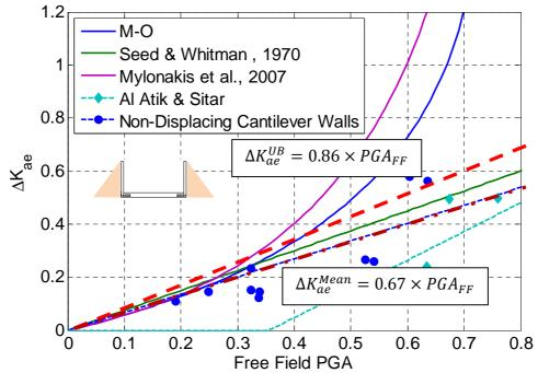
**Figure 7.3.** Back-calculated dynamic earth pressure coefficients at the time of maximum dynamic wall moments and maximum dynamic earth pressures on the non-displacing U-shaped cantilever wall as function of peak ground acceleration measured at top of soil in free field.
