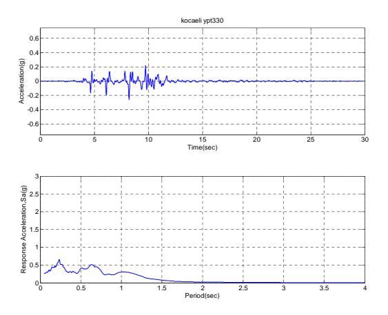
**Figure A.16.** Horizontal acceleration, response spectrum (5% damping) of Kocaeli-YPT330-1 input ground motion for ROOZ02.
