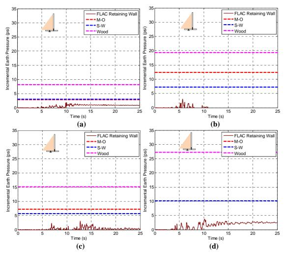
**Figure 5.23.** Incremental earth pressure time series computed by FLAC on Displacing Retaining wall during (a) Kocaeli-YPT330-1, PGA $_{\rm ff}$ =0.26 (b) LomaPrieta-SC-1, PGA $_{\rm ff}$ =0.62 (c) LomaPrieta-SC-2, PGA $_{\rm ff}$ =0.48 and (d) Kobe-TAK090-1, PGA $_{\rm ff}$ =0.87.
