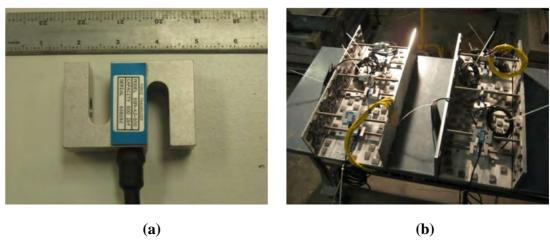
Figure 3.23. (a) Load cells, (b) Placed load cells between struts.
