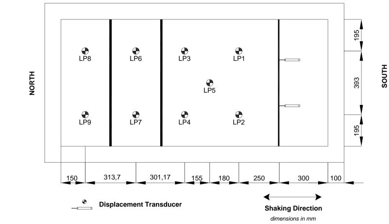
**Figure 3.6.** ROOZ02 model configuration, plan view (dimension in mm).
