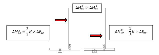
**Figure 7.4.** Effect of point of application of the seismic earth pressure increment on dynamic moment of retaining walls.
