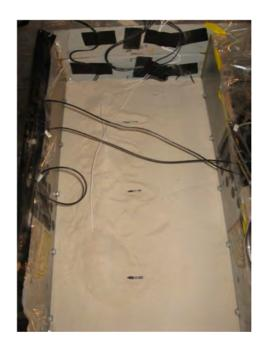
**Figure 3.13.** Placing accelerometers in the corresponding position.
