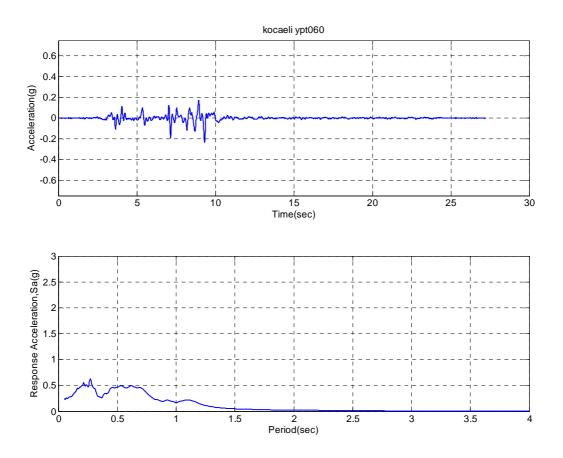
**Figure A.15.** Horizontal acceleration, response spectrum (5% damping) of Kocaeli-YPT060-3 input ground motion for ROOZ02.
