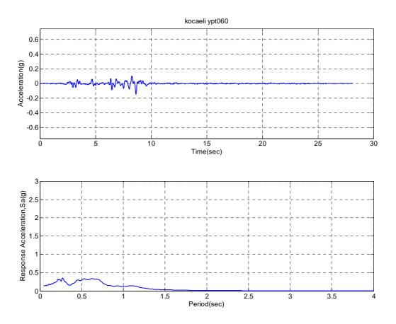
**Figure A.14.** Horizontal acceleration, response spectrum (5% damping) of Kocaeli-YPT060-2 input ground motion for ROOZ02.
