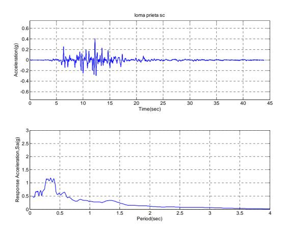
**Figure A.17.** Horizontal acceleration, response spectrum (5% damping) of Loma Prieta-SC-1 input ground motion for ROOZ02.
