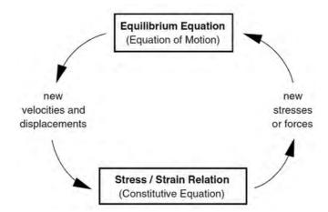
Figure 5.1. Basic explicit calculation cycle (from Itasca 2011).
