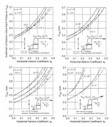
**Figure 2.4.** Comparison of active seismic earth pressures predicted by the solution proposed by Mylonakis et al. (2007) and from conventional M–O analysis, for different geometries, material properties and acceleration levels;  $a_v$ = 0 (from Mylonakiset al., 2007).
