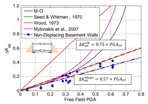
**Figure 7.1.** Back-calculated dynamic earth pressure coefficients at the time of maximum dynamic wall moments and maximum dynamic earth pressures on the non-displacing basement wall as function of peak ground acceleration measured at top of soil in free field.
