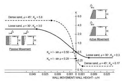
**Figure 6.13.** Effect of wall movement on earth pressure.
