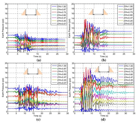
**Figure 5.19.** Total earth pressure time series computed by FLAC on South side of Non-Displacing Cantilever wall during (a) Kocaeli-YPT330-1,  $PGA_{ff}$ =0.26 (b) LomaPrieta-SC-1,  $PGA_{ff}$ =0.62 (c) LomaPrieta-SC-2,  $PGA_{ff}$ =0.48 and (d) Kobe-TAK090-1,  $PGA_{ff}$ =0.87.
