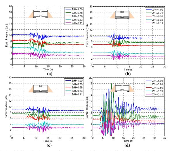
**Figure 5.16.** Total earth pressure time series computed by FLAC on South side of Flexible Basement wall during (a) Kocaeli-YPT330-2, PGA $_{\rm ff}$ =0.41 (b) Loma Prieta-WVC270-1, PGA $_{\rm ff}$ =0.49 (c) Kocaeli-YPT330-3, PGA $_{\rm ff}$ =0.51 and (d) Kobe-TAK090-2, PGA $_{\rm ff}$ =0.72.
