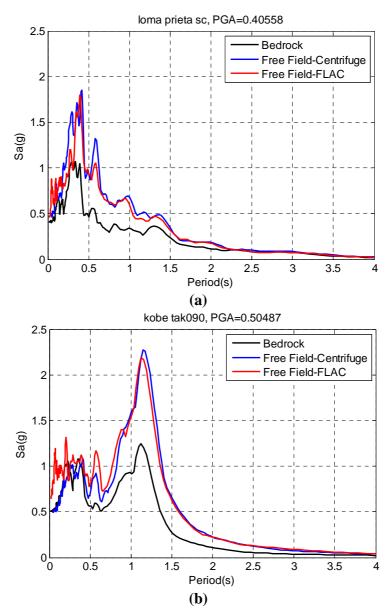
**Figure 5.8.** Comparison of recorded (centrifuge) and computed (FLAC) acceleration response spectra at 5% damping at the bedrock and top of the soil in the free field during (a) Loma Prieta-SC-1 and (b) Kobe TAK-090-2.
