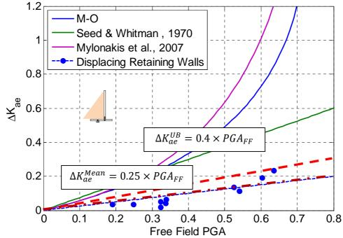
**Figure 7.2.** Back-calculated dynamic earth pressure coefficients at the time of maximum dynamic wall moments and maximum dynamic earth pressures on the displacing retaining wall as function of peak ground acceleration measured at top of soil in free field.
