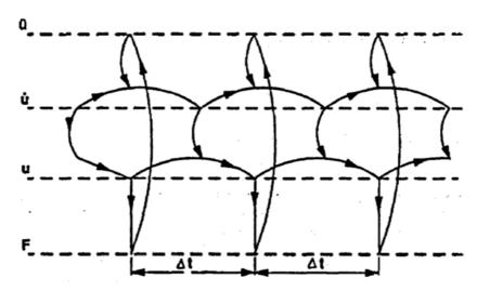
**Figure 5.2.** Interlaced nature of calculation cycle used in FLAC (from Itasca 2011).
