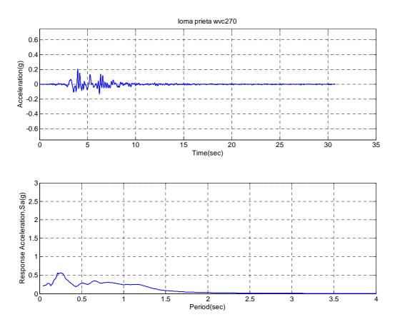
**Figure A.20.** Horizontal acceleration, response spectrum (5% damping) of Loma Prieta-WVC270-1input ground motion for ROOZ02.
