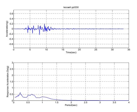
**Figure A.21.** Horizontal acceleration, response spectrum (5% damping) of Kocaeli- YPT 330-2 input ground motion for ROOZ02.
