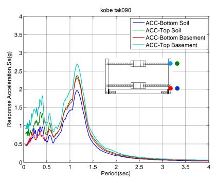
**Figure 4.8.** Spectral accelerations of top and bottom of the soil and the basement structure for Kobe-TAK090-2 event (5% damped).
