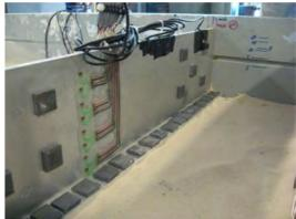
Figure 3.17. Strain gages located at the walls.
