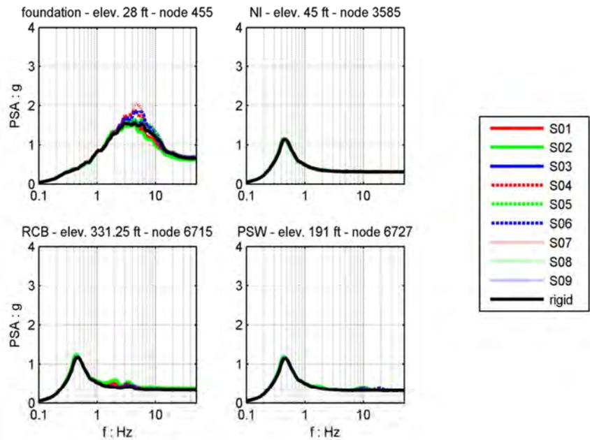
**FIG. 6. Pseudo-acceleration floor response spectra at different locations of the isolated structure for the different foundation soil conditions (median spectra of the 20 ground motions; X direction)**
