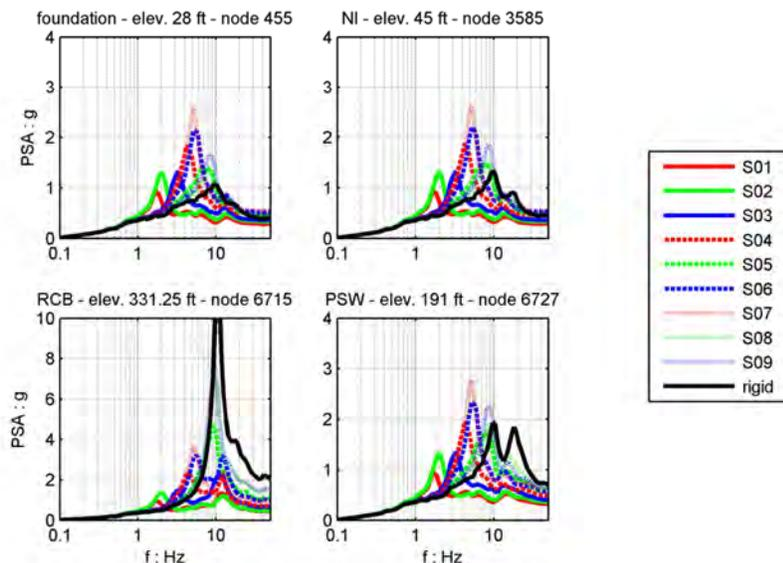
**FIG. 11. Pseudo-acceleration floor response spectra at different locations of the isolated structure for the different foundation soil conditions (median spectra of the 20 ground motions; Z direction)**
