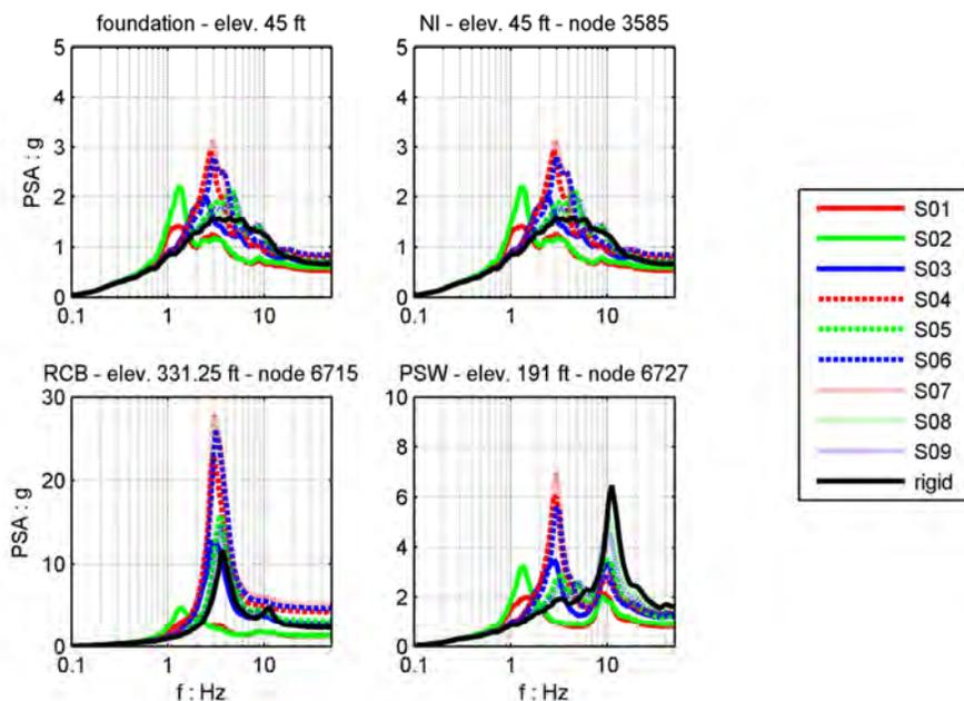
**FIG. 7. Pseudo-acceleration floor response spectra at different locations of the non-isolated structure for the different foundation soil conditions (median spectra of the 20 ground motions; X direction)**
