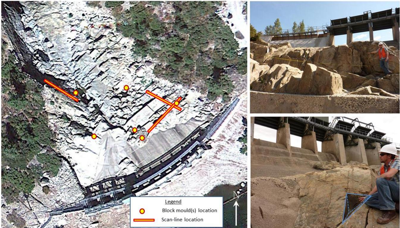
Figure 22: Scan-line survey and block mold locations (left), NE striking scan-line survey (upper right), block mold below spillway gate (lower right).
