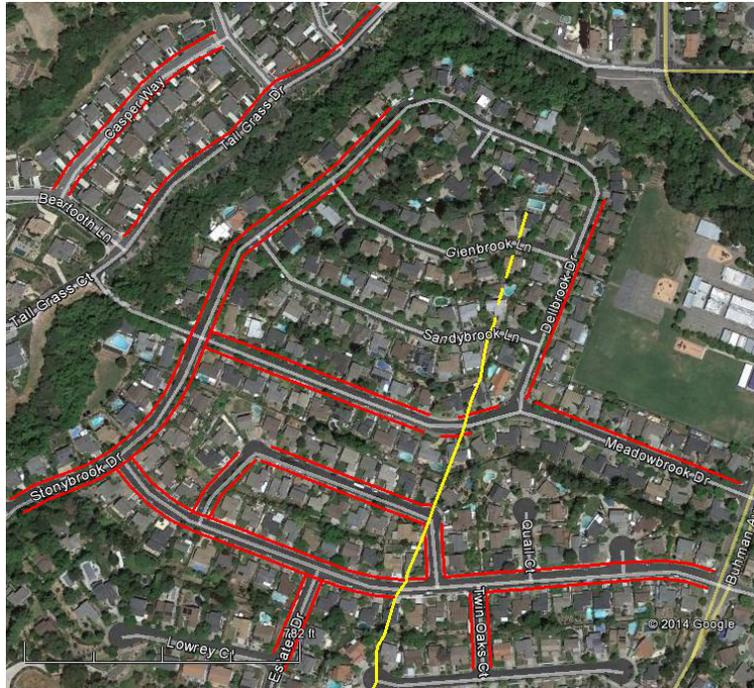
Figure 1: Observation and measurement sections of ground strain (red lines) and approximate observed fault trace (yellow line); produced in Google Earth; [Napa, CA; N 38.3040 W 122.3443; 8/26/14 - 8/28/14]; Bray et al. (2015).
