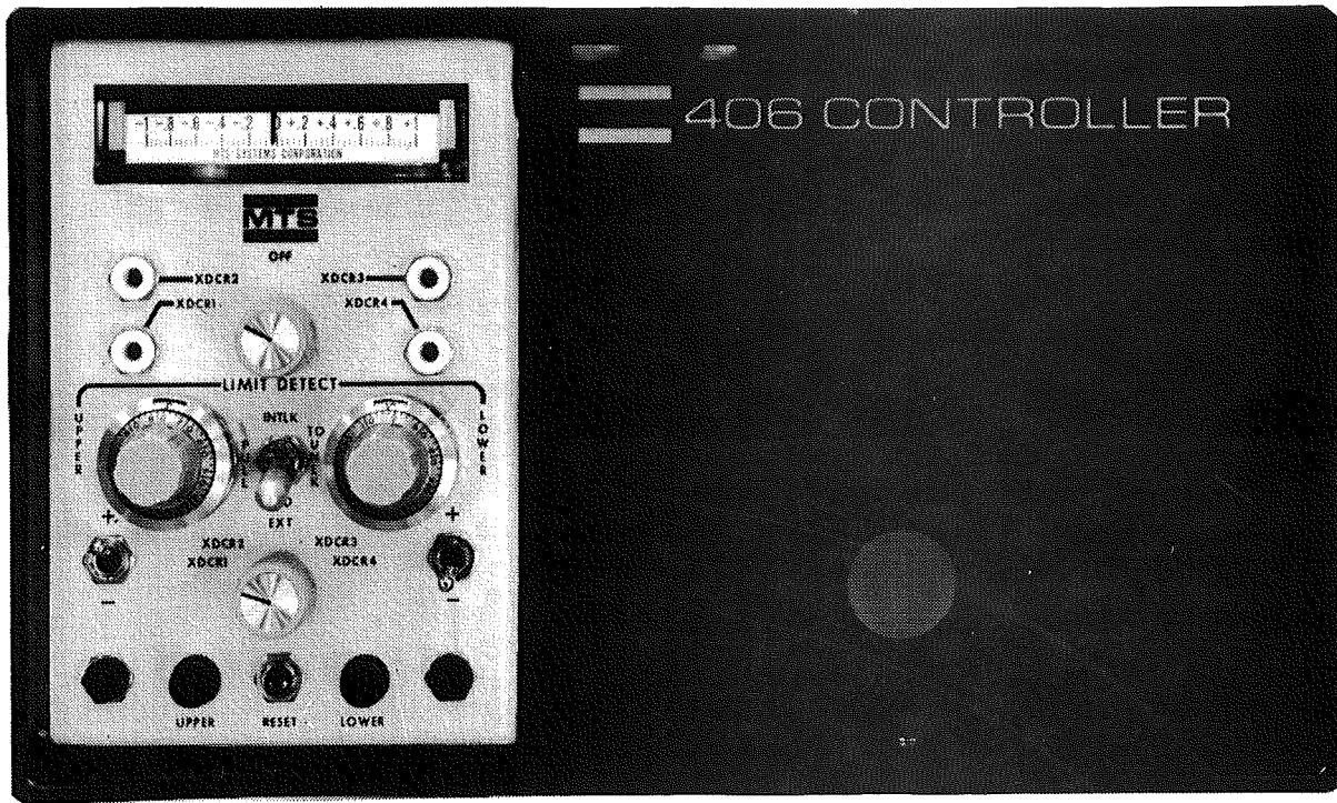
Figure 1-7. Conditioner Panel (Option F) Including Limit Detector (Option G)
